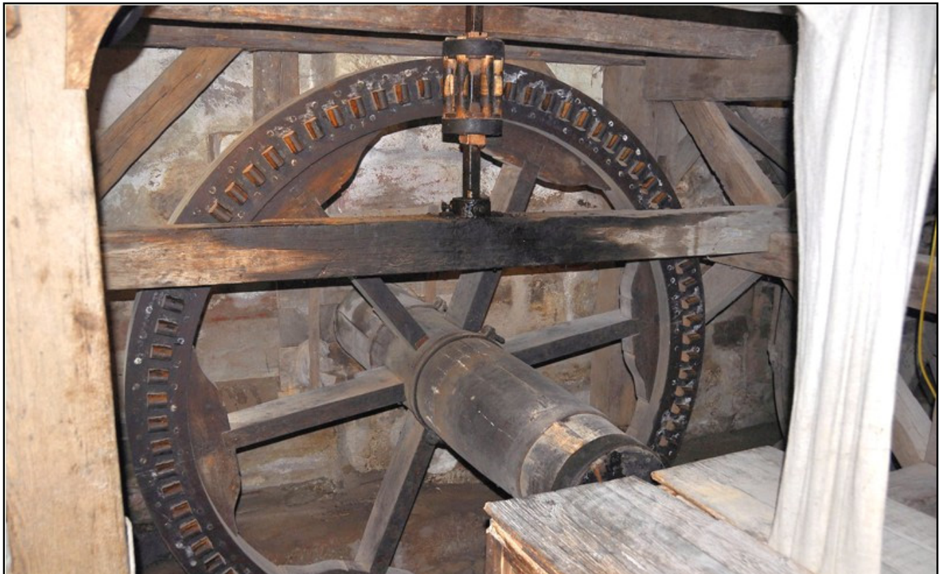
The Unterschlaubach Mill, above, the inner works, below, the main forward gear
